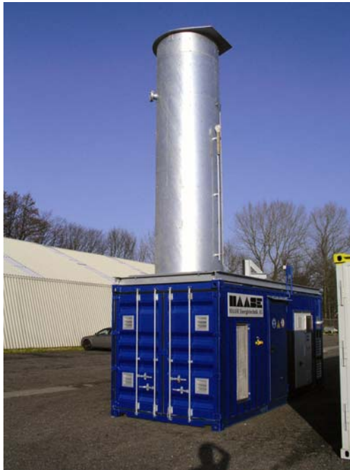
Picture 1: Mobile high-temperature flare for the disposal of explosive mixtures from tank farms. The total combustion capacity amounts to 5MW with a suction capacity from 500 to 3,000m 3 /h
